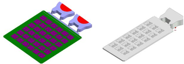
(a) Panel Solid Model (b) Panel Wire Frame Model
