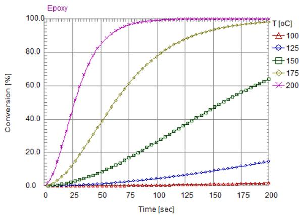
Fig 4. Curing Kinetics Curves: Conversion (%) vs Time
