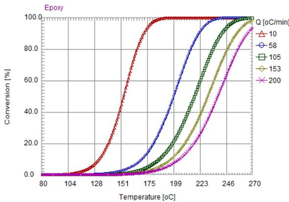
Fig 3. Curing Kinetics Curves: Conversion (%) vs Temperature
