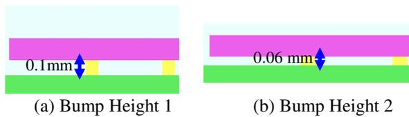
Fig 19: Void Locations for Different Bump Height
