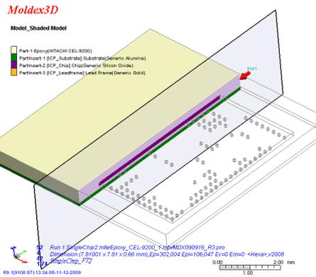
Fig 14: Cross Sectional Planar Cut for Analysis
