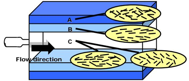
**Fig. 9** Simple sketch map of fiber orientation
