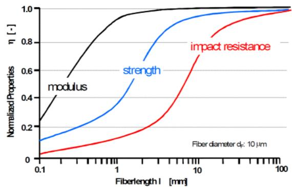
**Figure1.** Composite property improvement with increasing fiber length
