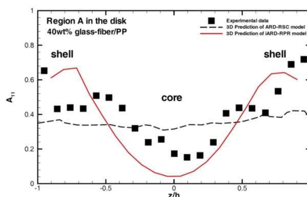
**Figure 2.** Moldex3D's long fiber simulation result (iARD, red line) shows an ideal agreement with observed data when compared to conventional ARD model (dotted line)
