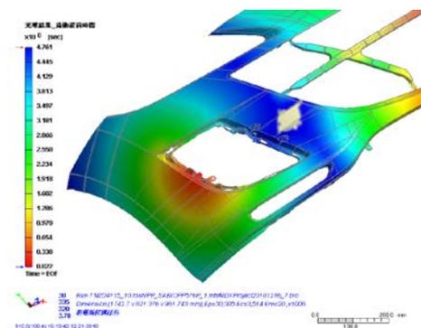
a. Prediction on air trap location opens for mold venting
