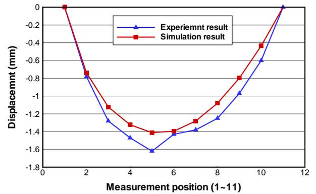
**Fig. 10** The comparison of deformation between experiment and simulation results
