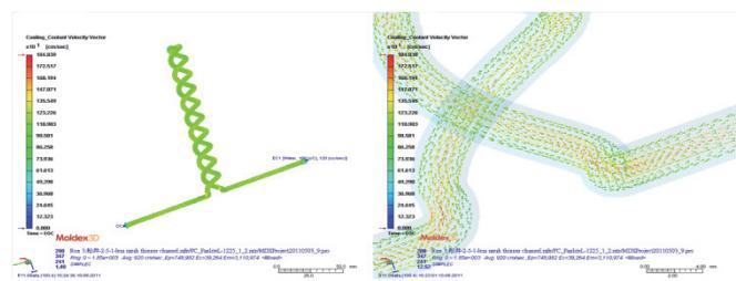
**Figure1.** Velocity vector inside a twin-spiral cooling channel
