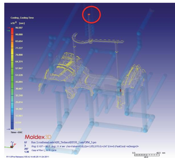
If we set the same temperature range for the two cases, we can see that conformal cooling channel effectively remove most of the heat from the core side. However, the max. temperature area still exists since no cooling channel pass that area (red circles).
