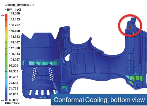
Below is the cooling efficiency comparison. In the conventional design, since the baffle does not reach the core side of the part, the lower cooling channel only absorbs 1/3 of the total heat. On the other hand, in the conformal cooling design, the conformal cooling channel has the highest efficiency (53.73), and conversely, the baffle cooling channel has a very low efficiency (1.16%).
