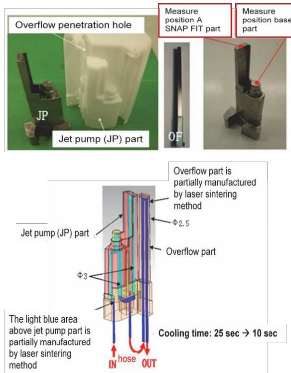
Figure 3 Auxiliary gas tank cooling improvement case
