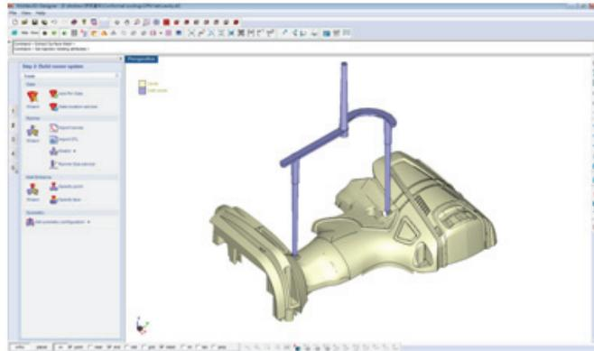
2. For the 3D cooling channels, just click the “import” icon. The supported file formats are .stl, .iges, and .stp. If the file is not a surface mesh file (i.e. .stl file), the program will extract the surface automatically. Remember to assign the attribute to “cooling channel”
