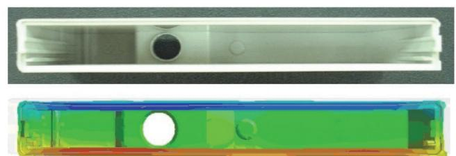
Fig. 5. Warpage results of revised design with conformal cooling –real injected part and simulation result
