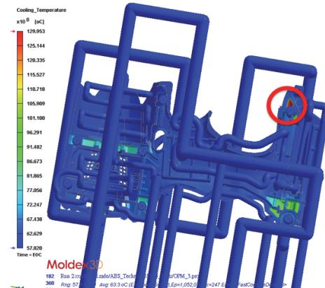
In terms of cooling time, the Max. cooling time required is also reduced to 96.51 seconds.
