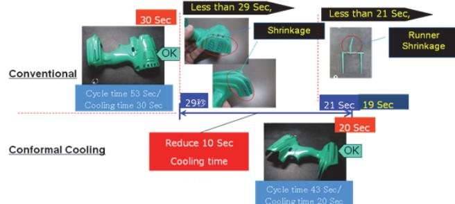
For instance, the sink mark can be used as an index for the product quality. Below are the sink mark comparison of the conventional design with 30 seconds cooling time and the conformal cooling design with 20 seconds cooling time. We can see that the sink mark values at the indicated areas are quite the same in these two cases (Normal: 0.07mm; Conformal: 0.08mm).
