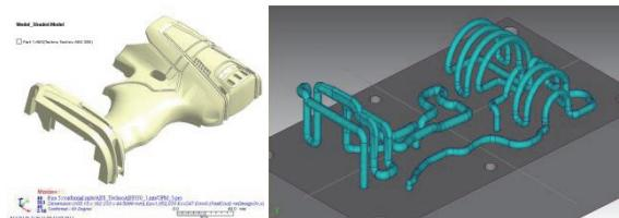
Figure 4 Machine tool cover model and conformal cooling design
