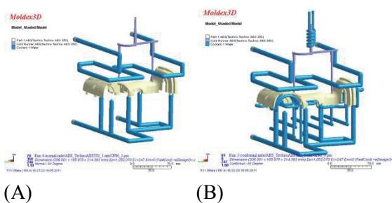
Figure 5 Conventional (A) and conformal cooling (B) design
