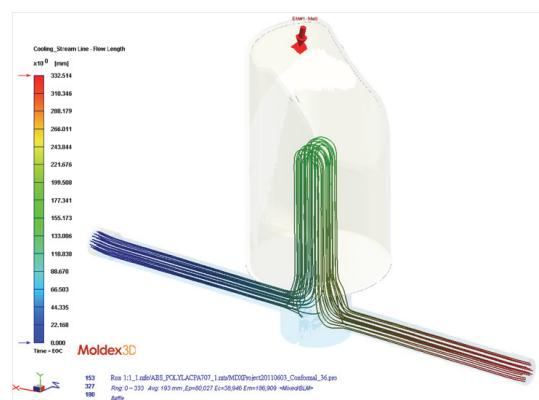
**Figure2.** Stream lines inside a baffle cooling channel
