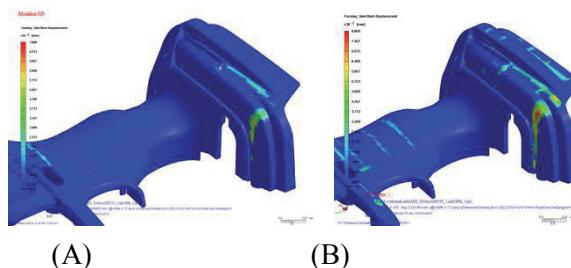
Figure 7 Sink mark displacement comparison
